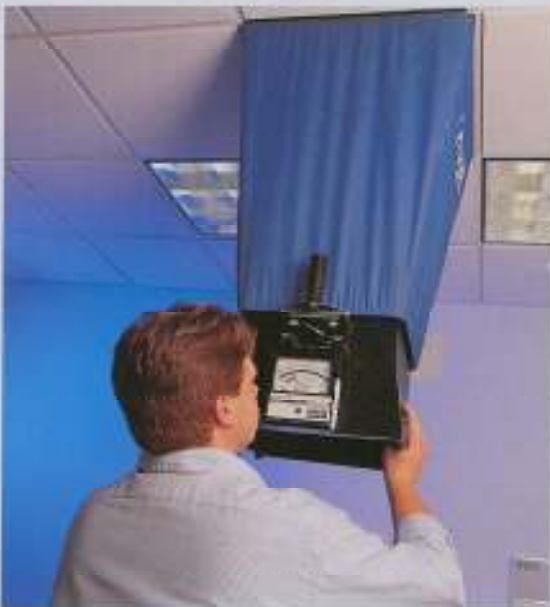
Don't put too much confidence in the hood measurement without taking the initiative to verify the accuracy.
